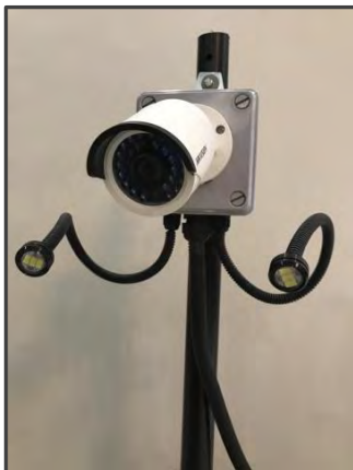
CCTV System complete with 2 No. LED lights
